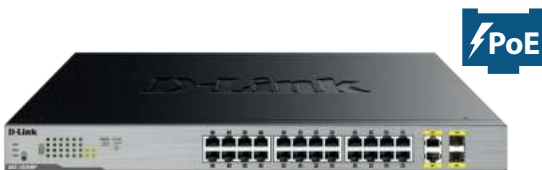
DGS-1026MP • 24 x 10/100/1000Base-T PoE ports PoE budget up to 370 W • 2 x 1000Base-T/SFP combo ports Dimensions: 440 x 250,4 x 44 mm
