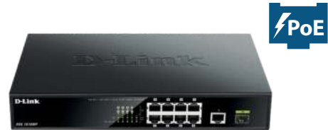
DGS-1010MP • 8 x 10/100/1000Base-T PoE ports PoE budget up to 125 W • 1 x 10/100/1000Base-T port • 1 x 1000Base-X SFP port Dimensions: 280 x 180 x 44 mm
